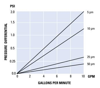
Flow rates exceeding 7-8 GPM per 10" length are not recommended for 50 microns or below for maximum service life. This chart represents the typical flow rate per 10" cartridge length. The test fluid is water at ambient temperature. Extrapolations for multiple lengths tend to be linear, but as flows increase the differential pressure across the housing becomes more apparent.
